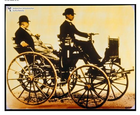
Source: Gottlieb Daimler with son Adolf in his first Vehicle with an Internal Combustion Engine (1.5 hp, 18 km/h)
